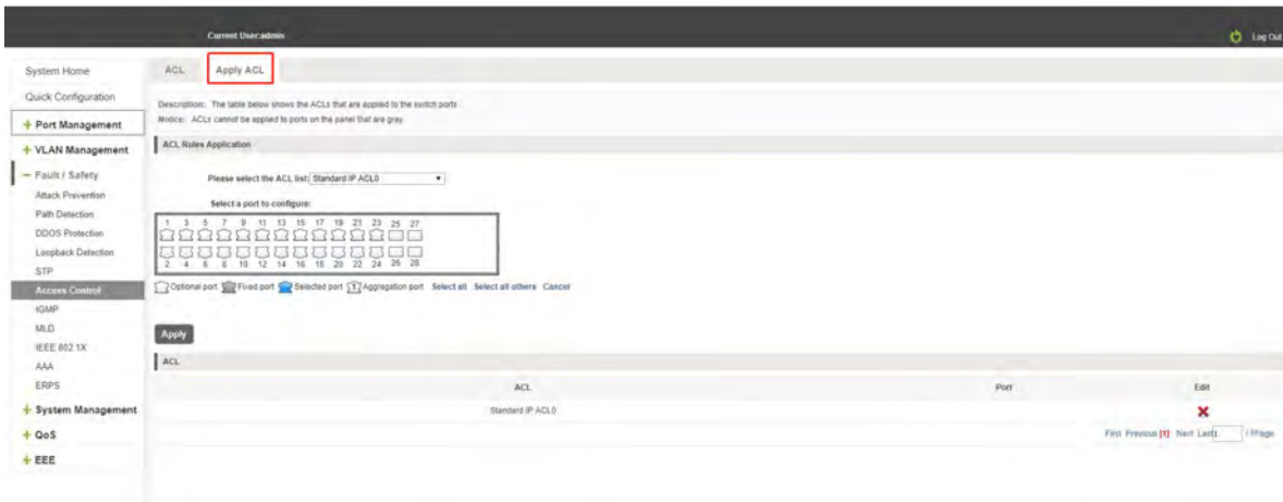
Figure 5-32: View application ACL rules
